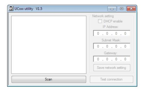
Press the 'scan' button to list the motion controller devices connected to the network. Doing so the software will send a broadcast massege to the network and will map all the available motion controller devices connected and running and will list the devices serial numbers in the listbox on the application form like this:
