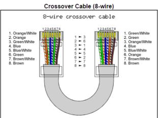
Use this cable for connection via router(s).
